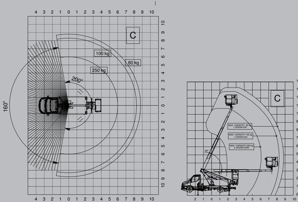
**CROSSBEAMS ONE SIDE FULLY OPENED ONE SIDE CLOSED**
