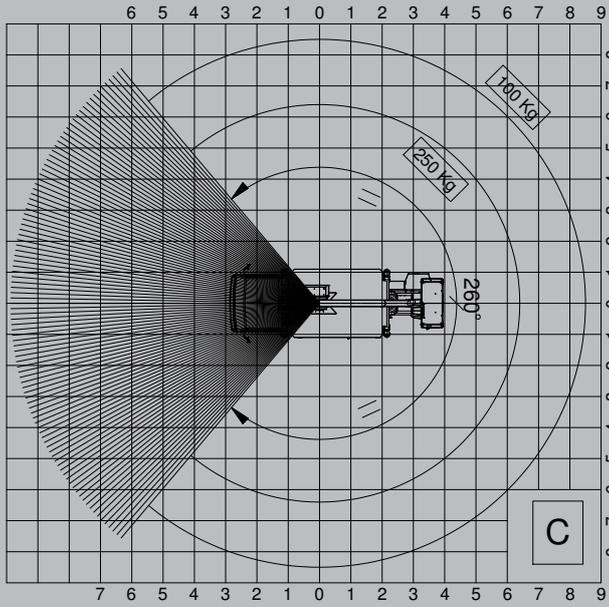
**CROSSBEAMS ONE SIDE FULLY OPENED ONE SIDE CLOSED**
